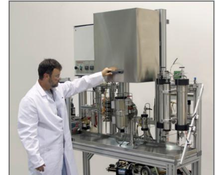
Core Flood Systems designed to meet specific applications as required by laboratories individual needs.
