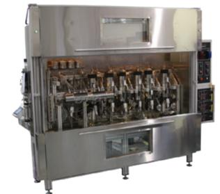
3-phase closed loop recirculation core flow system
